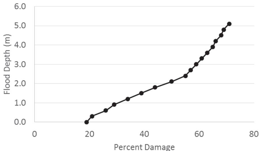
**Figure 3-2. Example of a flood depth-damage function (residential homes).**
