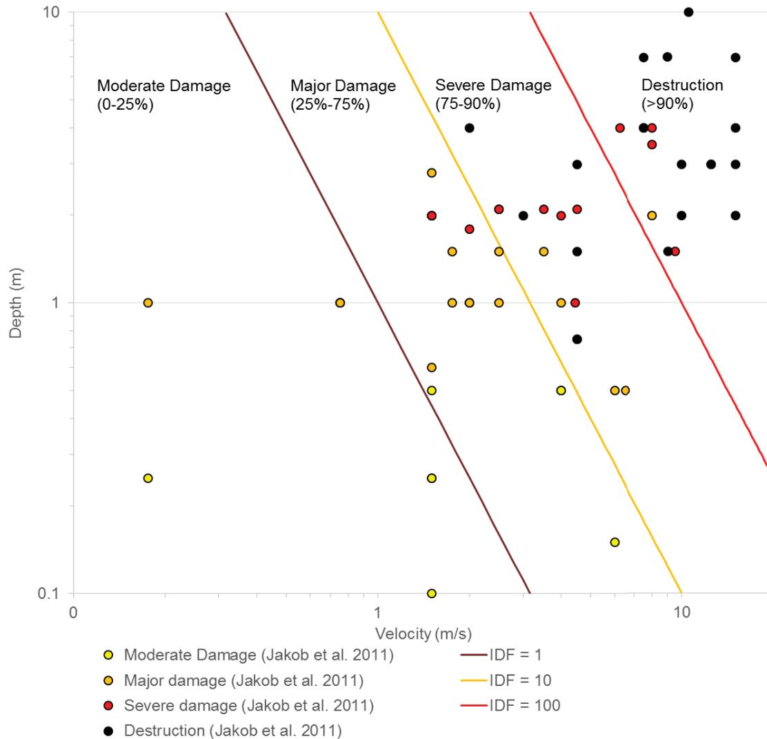
**Figure 3-3. Building damage cases reported by Jakob et al. (2011), plotted as a function of flow depth and velocity. Damage thresholds are plotted according to Equation [7].**
